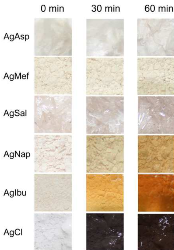
Figure 3: Reduction of synthesized silver(I) compounds in presence of high-energy UV radiation at 258 nm and 30 watts.
